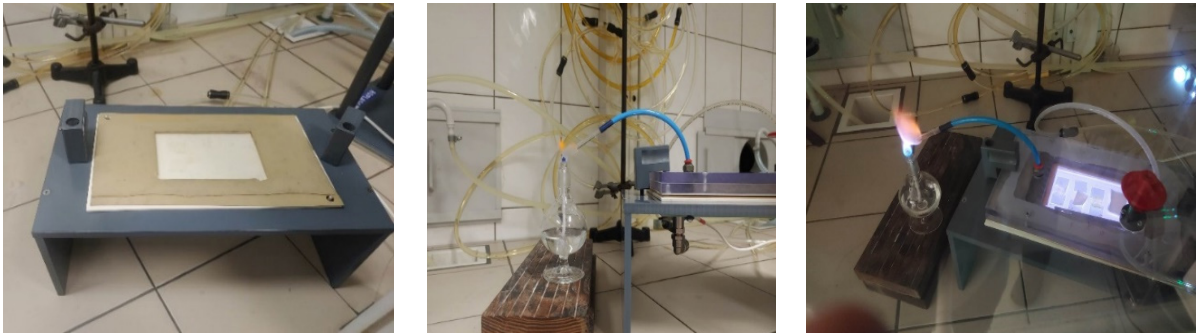
Figure 2. (a) Cold plasma equipment, (b) De-oxygen in the chamber, and (c) Cold plasma stabilization process Wettability measurement by the sessile drop method
